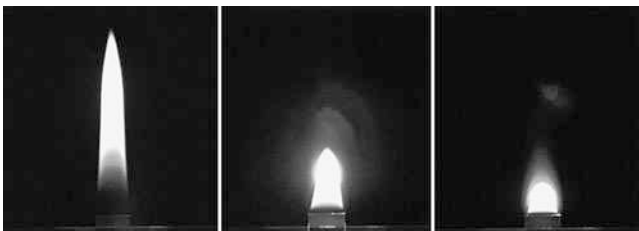
Fig. 7.5 Natural gas diffusion jet flames surrounded by different gas mixtures: Left: air; Middle: 50% oxygen/50% nitrogen; Right: 100% oxygen (Reproduced with permission from Lee et al. [3])
